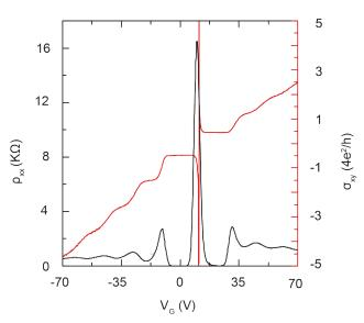
Characterisation indicating high-quality, defect-free graphene produced using a nanoCVD-8G. Left: Raman spectrum. Right: Longitudinal resistivity and Hall conductance data indicating half integer quantum Hall effect unique to monolayer graphene (data taken from reference 1).
