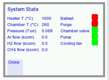
Screen shots from the touch screen HMI software through which all user operation of the nano CVD-8G is carried out.
