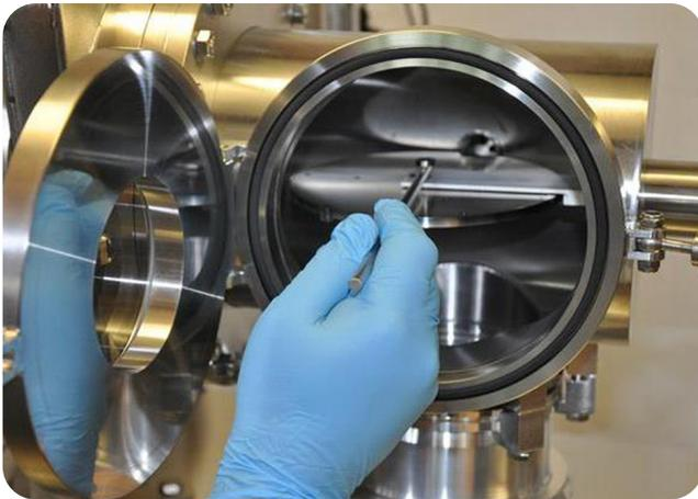
Inserting substrates into a MiniLab 125 load-lock
