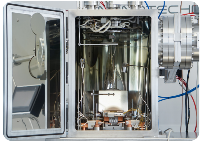
Process chamber configured for e-beam evaporation with optimised working distance
