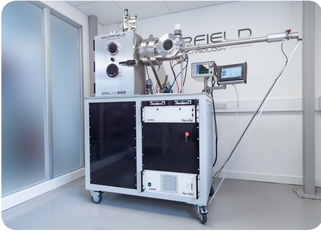
Moorfield MiniLab 080 system for e-beam evaporation with automatic process control and load-lock
